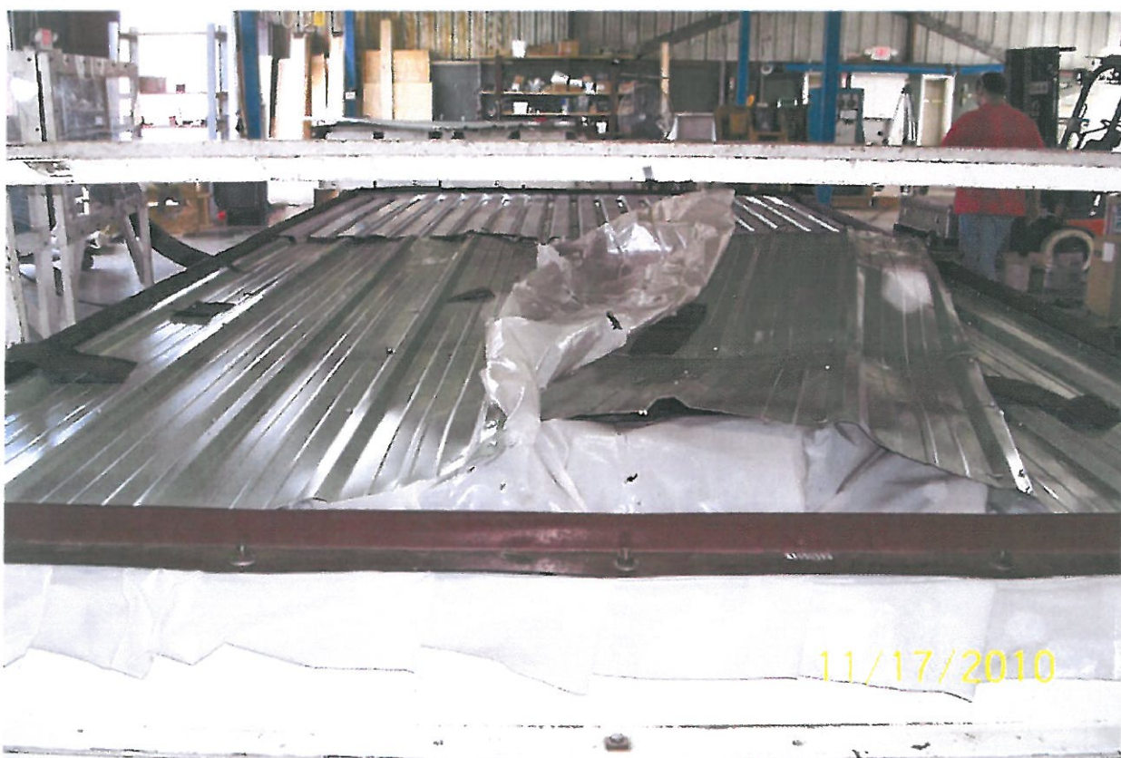
TEST B FAILURE: PANEL PULLED OVER FASTENER
