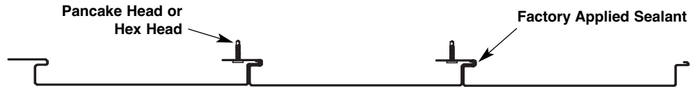
Typical Seam Engagement Pancake Head or Hex Head Fastener (Fastener Type as Required)
