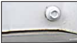
Environmental tests show extensive corrosion along cut end of panel without Edge-Rust Inhibitor.
