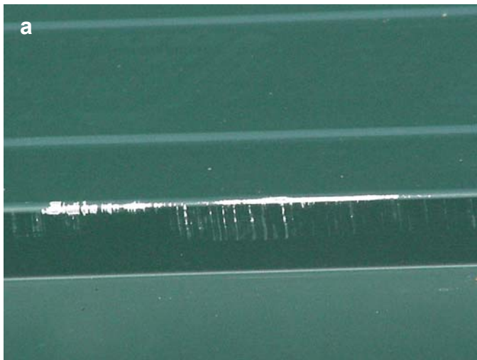
Figure 9. Photographs of paint abrasion damage on the major rib of the panel (a), and scratches on the surface of a painted panel resulted in premature corrosion (b).
