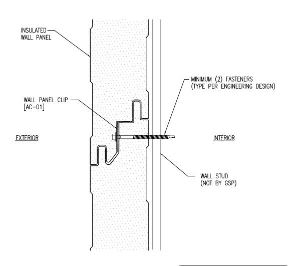
3/8" UNIFORM BEAD OF NON-SKINNING BUTYL SEALANT MUST BE APPLIED IN EITHER OR BOTH FEMALE GROOVES DEPENDING ON VAPOR SEAL REQUIREMENTS
