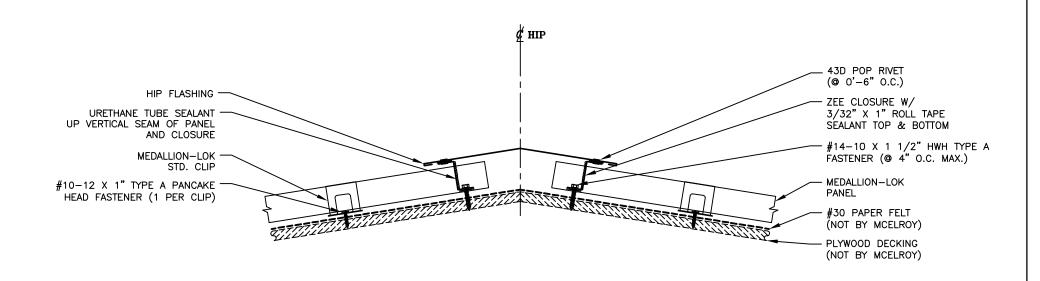
INSTALLER NOTE: TEMPORARY FASTENER MAY BE REQUIRED TO KEEP PANELS FROM SLIDING DOWNHILL DURING INSTALLATION.
