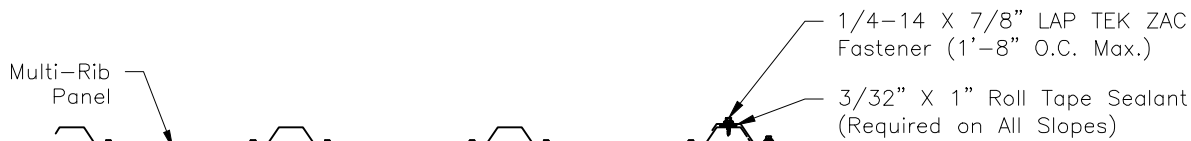
FASTENER PATTERN (@ Eaves, Ridges & Endlaps)
