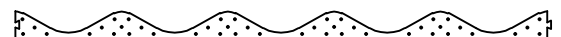
FOAM INSIDE/OUTSIDE CLOSURE (Plugs in closure can be removed to allow for ventilation)
