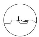
**WAVE FLOATING SEAM ENGAGEMENT** WAVE FLOATING UTILIZES SEPARATE CLIPS (SUBSTRATE & FOAM CLOSURES NOT SHOWN FOR CLARITY)
