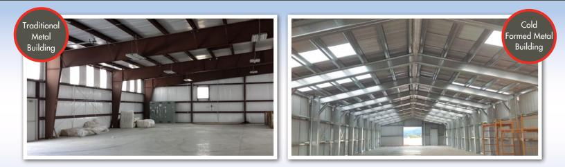
**Aesthetically Appealing!** The dark red paint commonly used for traditional metal buildings offers poor light reflectivity. In contrast, we use Galvanized material in our Cold Formed Building line which provides a clean and bright appearance.
