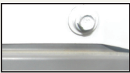
Minimal corrosion is detected along cut end of panel with Edge-Rust Inhibitor application.
