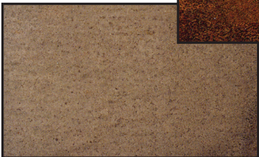
To the right: Galvanized test panel covered in red rust after 18 years in a rural environment
