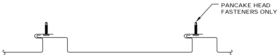
FW SERIES CUSTOM REVEAL SEAM ENGAGEMENT
