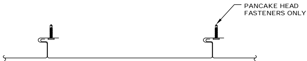
FW SERIES TYPICAL SEAM ENGAGEMENT
